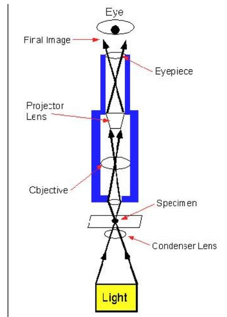
**Figure 1.1:** Basic principle of a light microscope or optical microscope.
