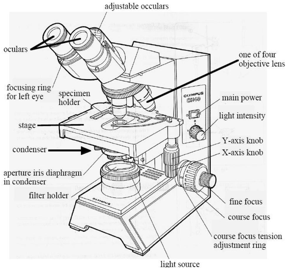
**Figure 1.2:** Different parts of a compound light microscope.
